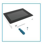
Using a small flat-blade screwdriver to insert it into the empty slot at the front cover. Then use the screwdriver to pry the thermostat forward, and then please separate the front cover from the back cover by hand carefully.
