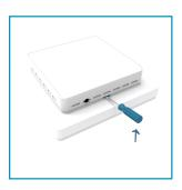
Using a small flat-blade screwdriver to insert it into the empty slot at the bottom of the cover frame that is in contact with the front cover. Then use a screwdriver to pry the thermostat forward, and then please separate the front cover from the back cover by hand carefully.
